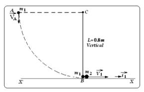
Just after collision  $m_2$  moves with velocity  $\overrightarrow{V_2}'$ , of magnitude 2m/s,  $(\overrightarrow{V_2}'=2\overrightarrow{\iota})$  and  $m_1$  moves with velocity  $\overrightarrow{V_1}'$ . Neglect air resistance. Use  $g=10m/s^2$ .
